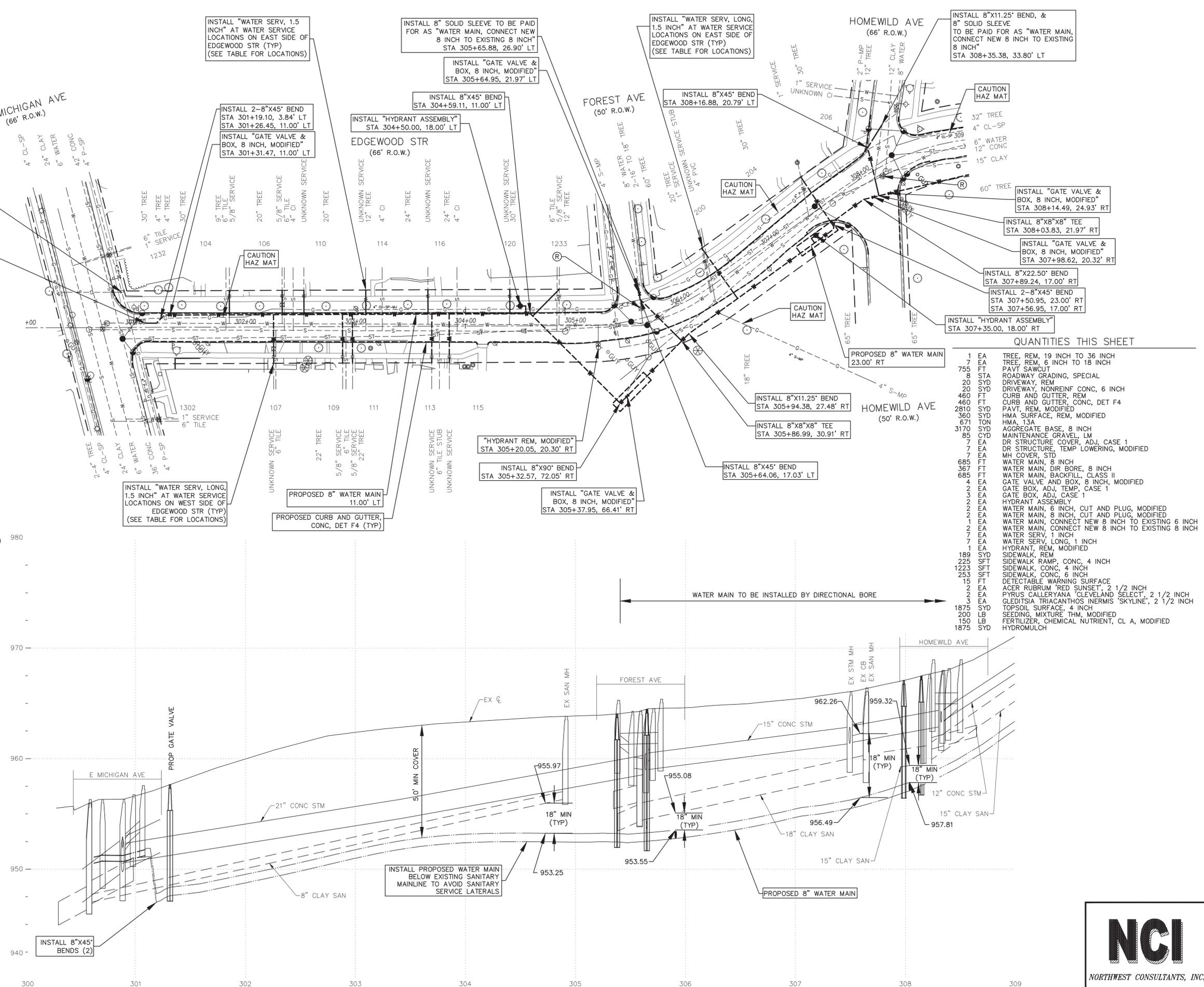
INSTALL 8"x6" REDUCER, 6" DI PIPE & 6" SOLID SLEEVE TO BE PAID FOR AS "WATER MAIN, CONNECT NEW 8 INCH TO EXISTING 6 INCH" STA 301+09.10, 3.84' LT
